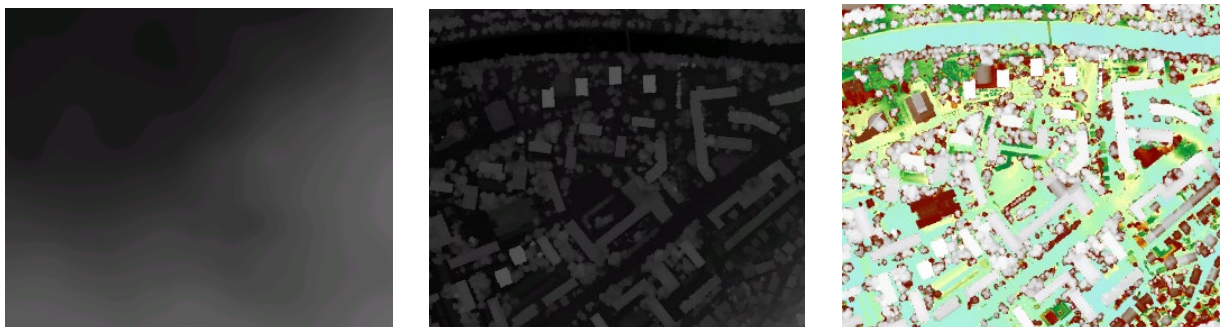
From left to right: DTM, DSM, nDSM
