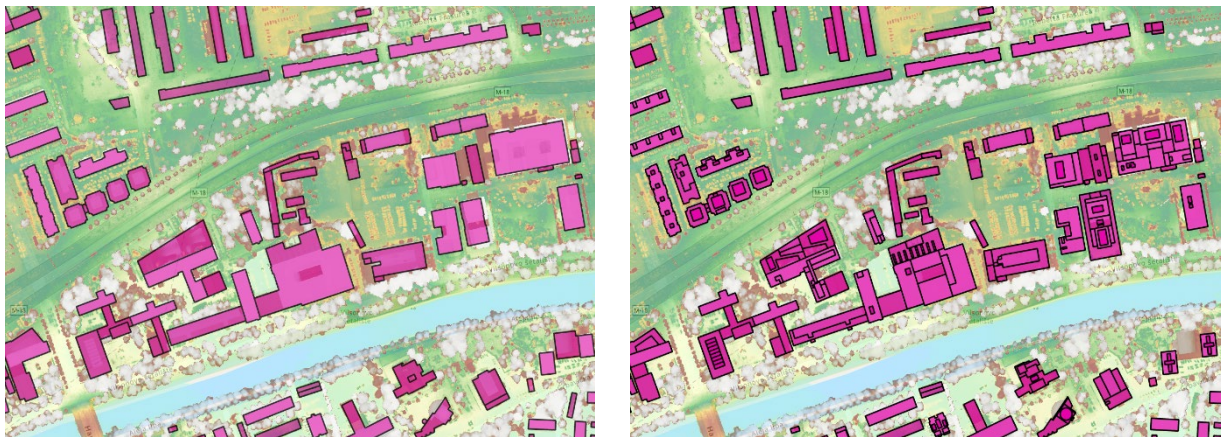
Left: Buildings with lower level of detail; Right: Segmented buildings with higher level of detail
